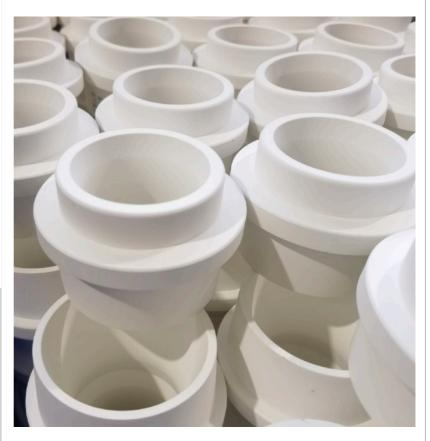
Sprue bush is also known as insulating sleeve. It is a part on the low pressure casting machine for alloy wheel and other similar casting. Sprue bush is used to form low pressure runner.
