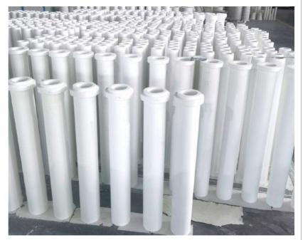
The aluminum titanate ceramics with high melting point, low thermal expansion coefficient, low thermal conductivity, and excellent thermal shock resistance and corrosion resistance. It is the best thermal shock resistance among low-expansion ceramics. The aluminum titanate has excellent high temperature resistance and can be used for a long time at 1400°C. It is mainly used in special environment with dramatic change in temperature and strong corrosion.
